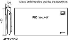
It is recommended to keep the distance of 150 mm between the convector and the floor of the room.
