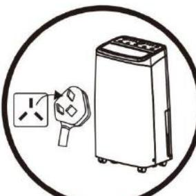
Do not turn off the dehumidifier directly with the power switch. Turning off the dehumidifier with the power switch may result in electric shock, fire, etc. Always use the control panel to stop the dehumidifier operation. Turn off the power switch when not in use for a long time. Dust accumulation may cause leakage, loss, heat, fire, etc. Turn off the power to avoid lightning strikes.
