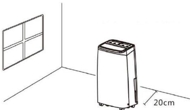
When the dehumidifier is working, make sure that the minimum clearance at the rear is 20cm, as shown.
