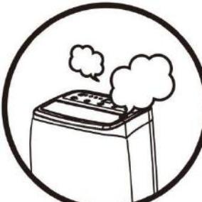
When an abnormal phenomenon (such as a burnt smell) occurs, the operation must be stopped and the power supply turned off. Continued use may result in malfunction, electric shock or fire. Please entrust your local dealer or service outlet for repairs.
