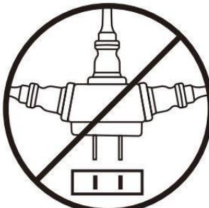
It is forbidden to replace the power cord without authorization, or connect the power cable in the middle and other appliances in parallel. Unauthorized replacement, mid-way connection, overload use may cause electric shock or fire. If the power cord is damaged, please entrust your local dealer or service outlet for repair.
