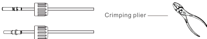
Pic 3.4 Crimp the contact pin to the wire
